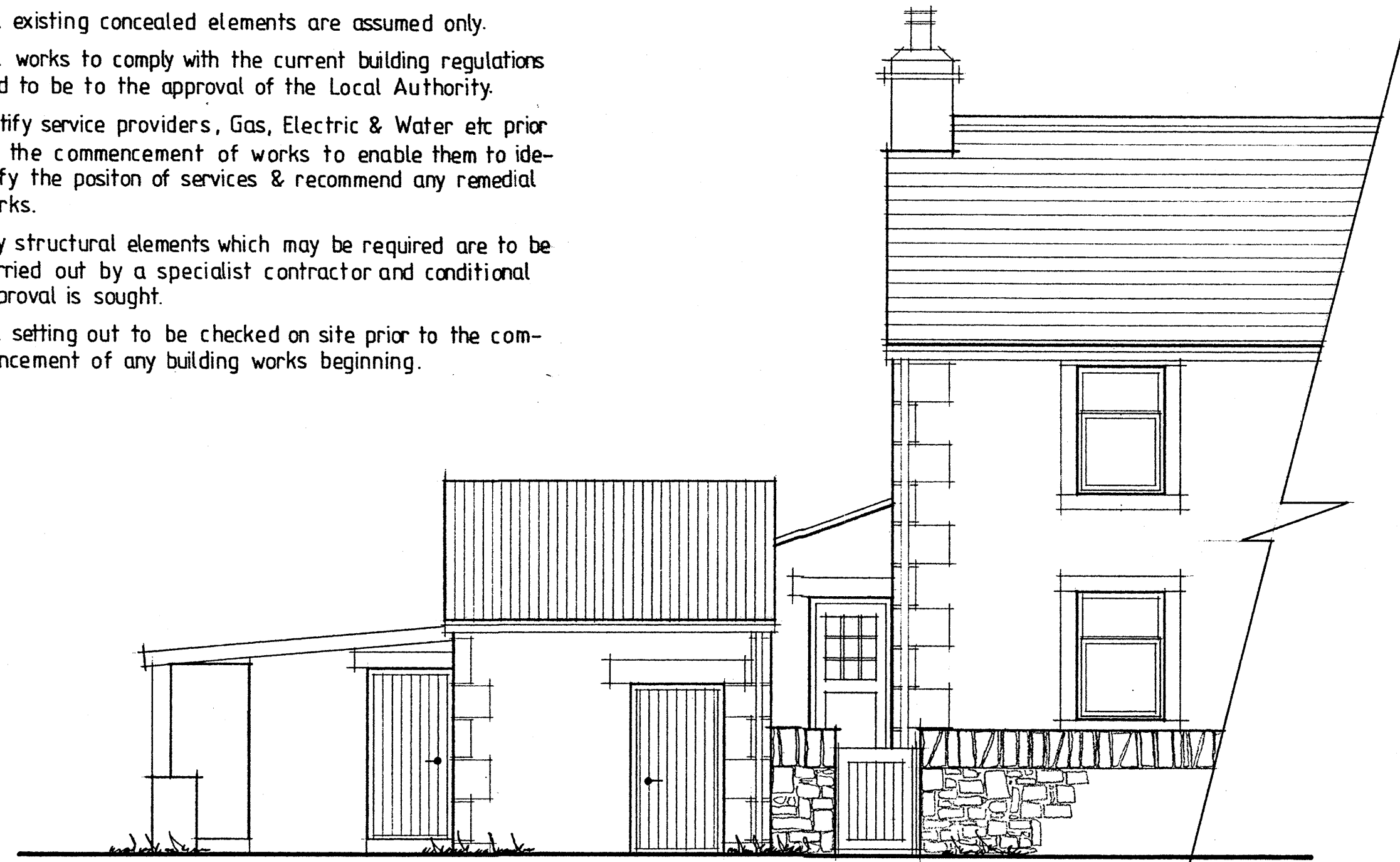
West Elevation as existing 1:50
